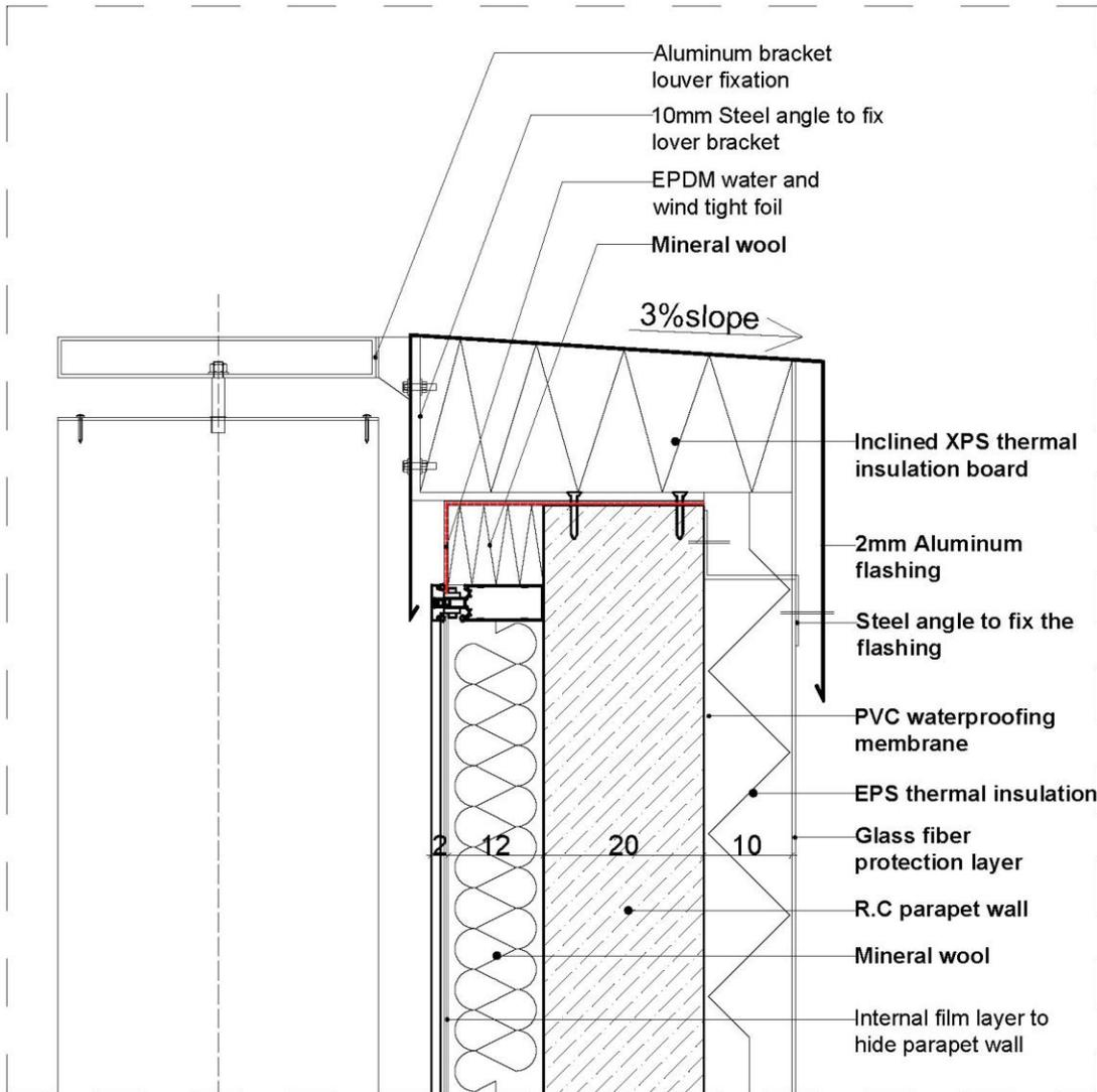
Parapet wall with louvers connection detail
