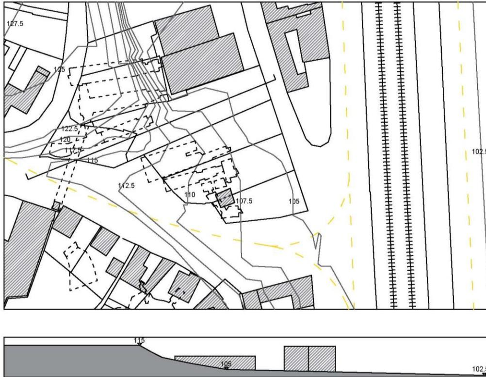
Slope difference up to 10 meters between the lower and the upper street
