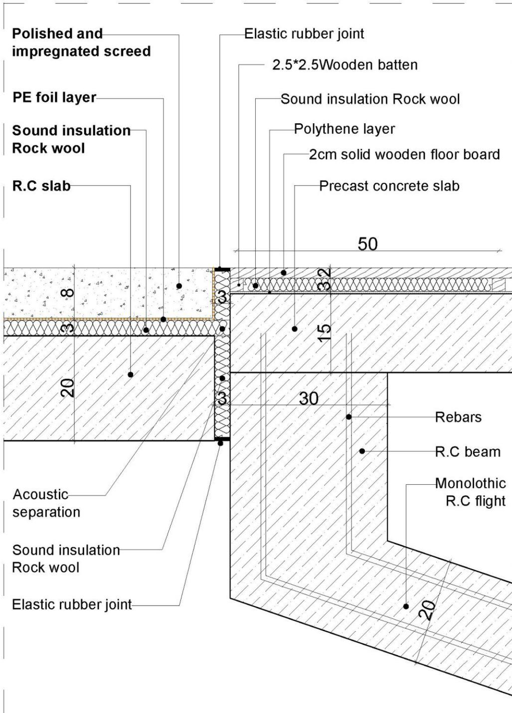
Auditorium with first floor slab connection detail
