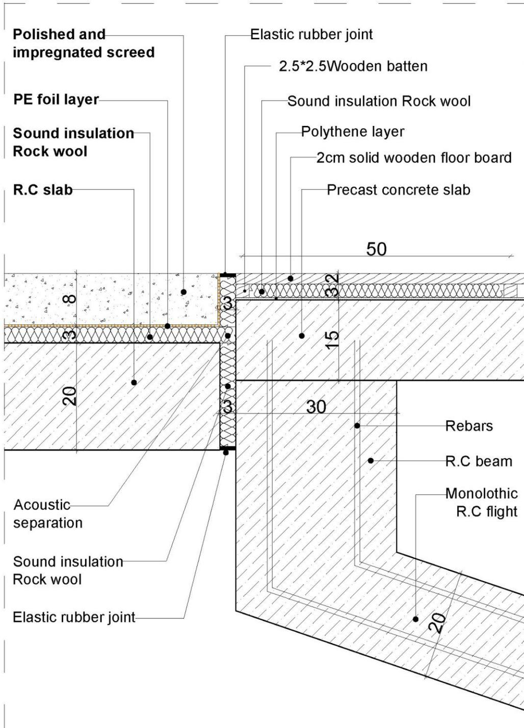
Auditorium with first floor slab connection detail
