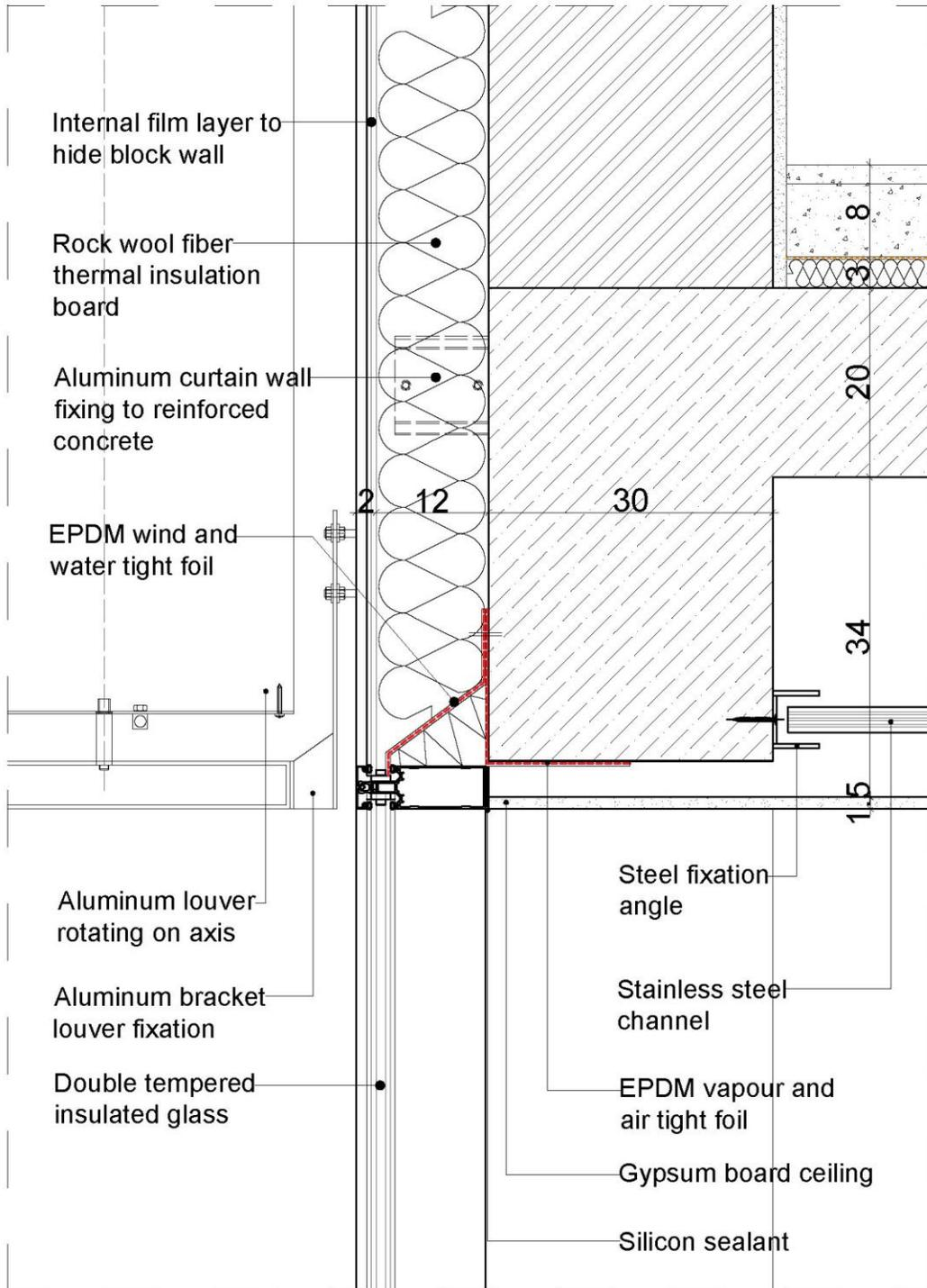
Curtain wall connection with beam detail
