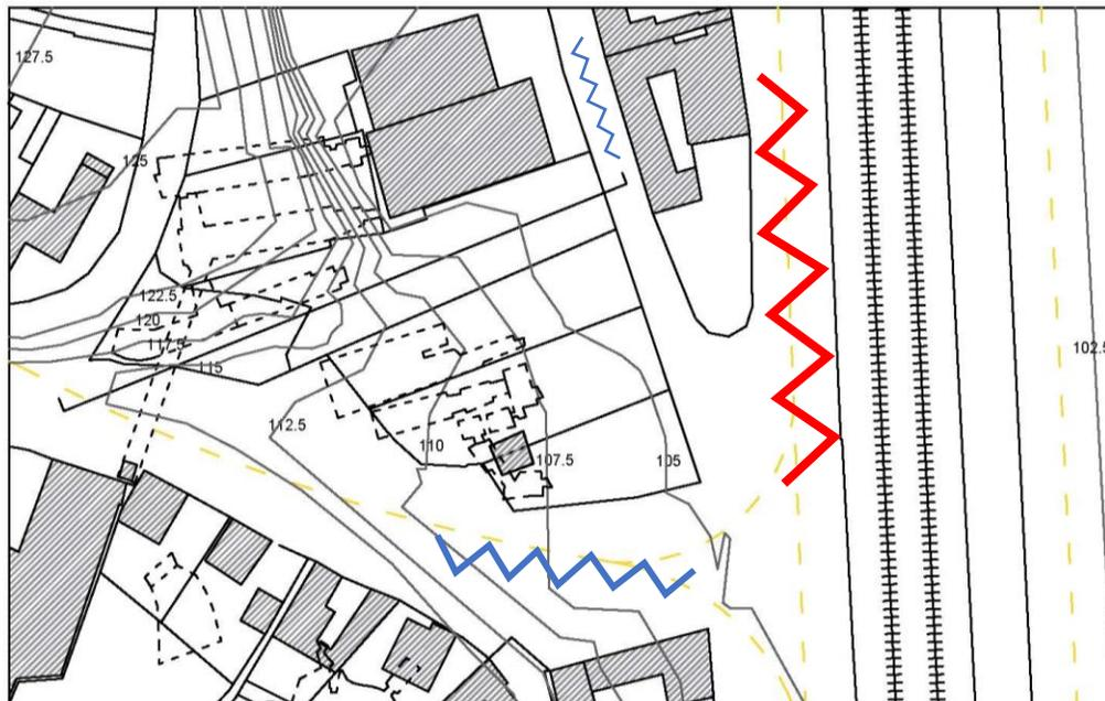
Most of the noises come from road 6 which has the railway as indicated on the drawing above, in this case noise level can reach 65-70 db and the allowed noise level for offices shouldn't exceed 40 db. Meanwhile, on Tóth József junction the site receives a little bit noise from cars passing daily to the residential area there. As mentioned before Kossuth Lajos street will be transformed to pedestrian road only according to Budafok development traffic plan.
