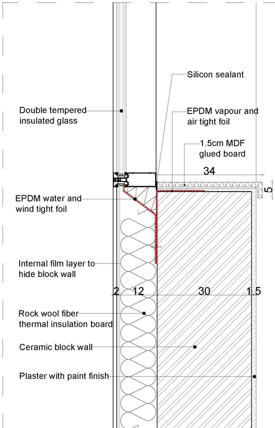
Curtain wall connection with block wall bottom detail
