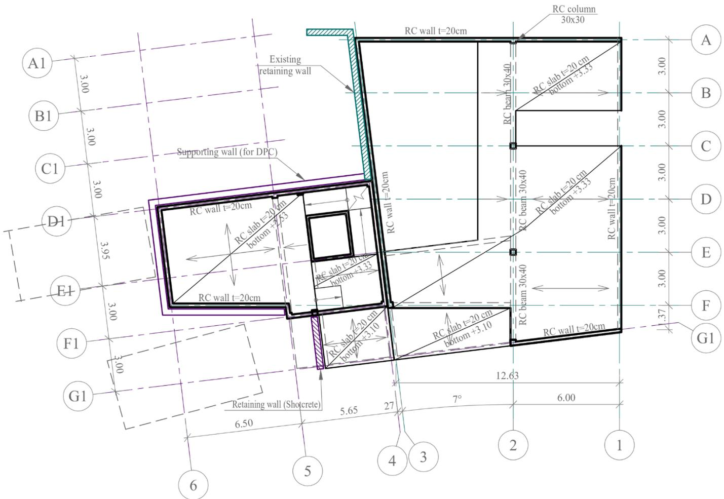
Reinforced concrete slab – thickness 20 cm – supported by reinforced concrete walls (20 cm) and columns (30x30 cm) + beams (30x40 cm). (see Figure 1<sup>st</sup> floor M1:200)
